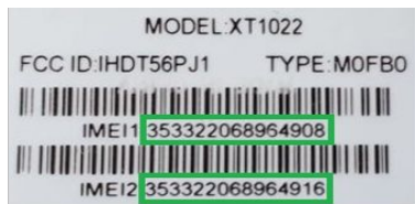
(a) Original and forged IMEI numbers created using copy-paste operations are marked by a green and red color, respectively.
