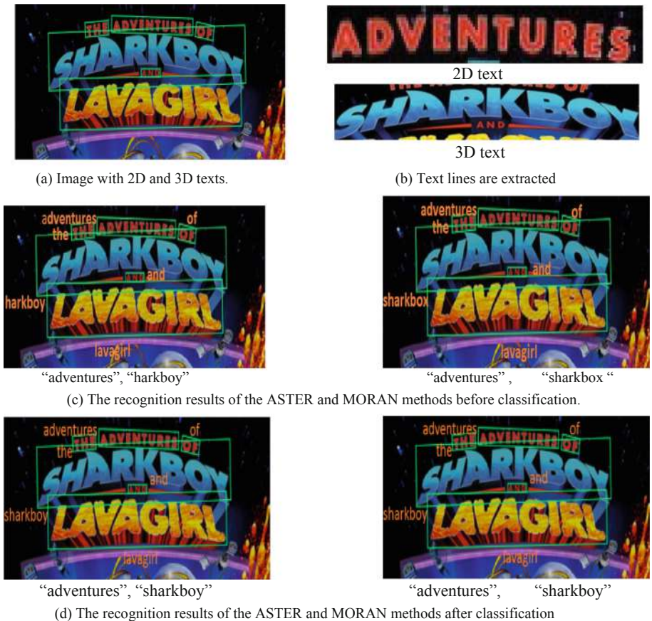
Fig. 1. Example of recognition results for 2D and 3D text before and after classification. The recognition results are displayed over the images for respective methods.
