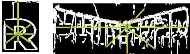
(b) Traversing in 360 directions to find stroke pixels for each connected component. Yellow color denotes direction and red pixel denote stroke pixels.
