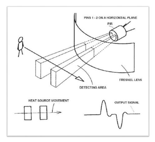
The IR sensor itself is housed in a hermetically sealed metal can to improve noise/temperature/humidity immunity. There is a window made of IR-transmissive material (typically coated silicon since that is very easy to come by) that protects the sensing element. Behind the window are the two balanced sensors.
