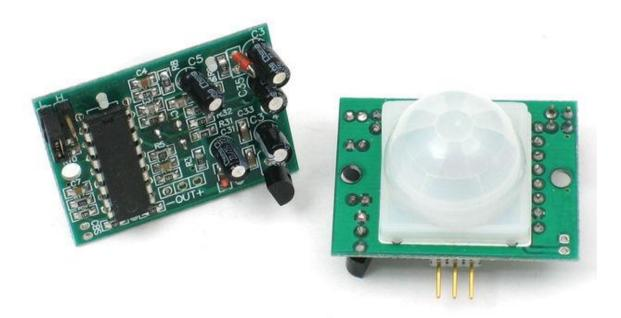
PIR motion detection sensor module
